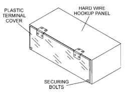
Figure 12. Plastic Face Plate (Output Terminal Lugs)
